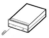
3. Press the front of the tray or lightly and gently pull the tray out with two fingers.
